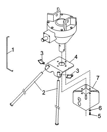
The Parking Stand Kit has a plate that bolts to the bottom of the gearbox. Two removable legs go into sockets welded on the plate. The legs are pinned in place. The two legs and the auger form a tripod which supports the post hole digger in a vertical position. A formed hook keeps the PTO driveline end off the ground.
