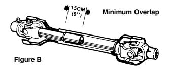
Apply multi-purpose grease to inside of outer (female) driveline section. Assemble driveline and install on tractor and digger. Check each driveline section to be sure yokes are "locked" to tractor and gearbox shafts. Make certain driveline shielding is in place and in good condition.
