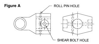
On the implement end of the PTO shaft there is a hole in the yoke just forward of the 3/8" shear bolt (see Figure A). This hole is for the 1/4" diameter x  $2^1/4$ " long roll pin (Ref. #21). When this roll pin is driven in this hole, the center of the roll pin engages into the groove on the front of the gearbox input shaft. This prevents the PTO assembly from coming off if the 3/8" shear bolt should shear.
