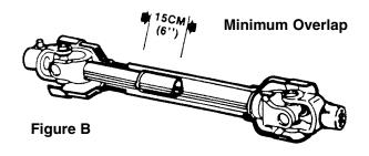
Apply multi-purpose grease to inside of outer (female) driveline section. Assemble driveline and install on tractor and digger. Check each driveline section to be sure yokes are "locked" to tractor and gearbox shafts. Make certain driveline shielding is in place and in good condition.
