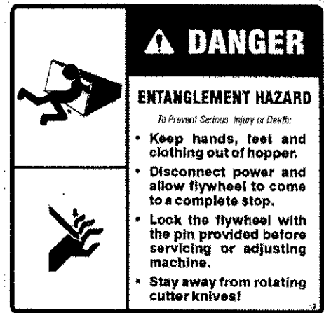
DECAL # 13 Location: Hopper extension (both exterior sides)
