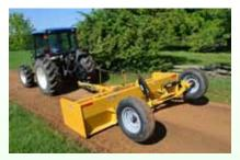
Available in three models 8', 10', 12' Constructed of 4" square tubing, 1/4" thick moldboard, 3/8" thick end plates 1/2" x 6" reversible cutting edge **Tilting ability** Includes hydraulic cylinders and hoses
